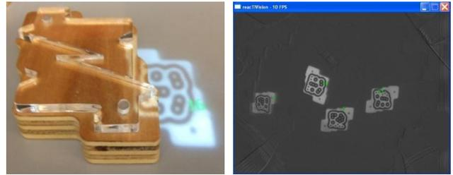
Figure 6. The IR camera identifies the fiducial tag.
