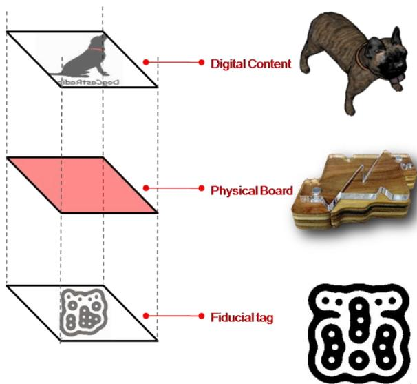
Figure 5. Each puzzle piece consists of three parts.
