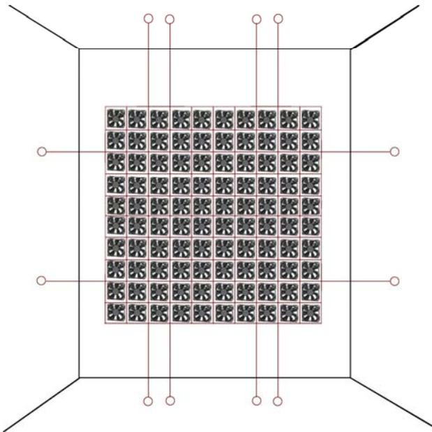
**Figure 8. Initial concept sketch of a grid of 10x10 fans suspended in a space.**
