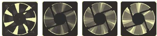
**Figure 5. Stroboscopic motion of fans speeding up and slowing down**
