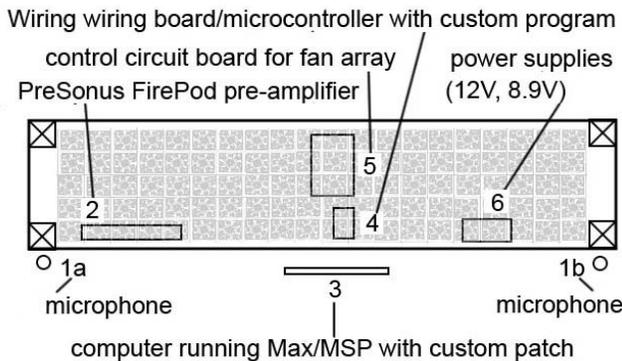
**Figure 3. Internal component layout**
