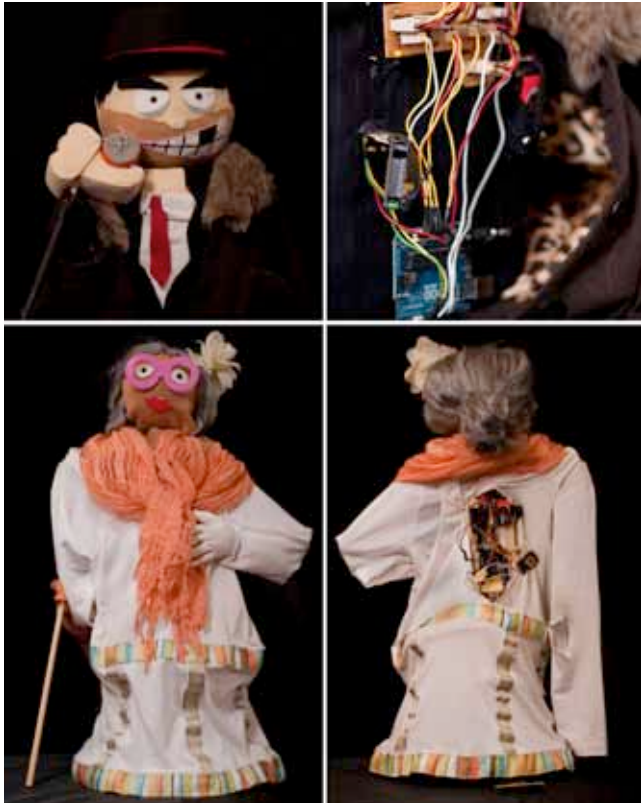
Figure 2. Front view of gangster puppet (top left) and electronics housed under his coat (top right). Front view of old lady puppet (bottom left) and electronics housed in her back (bottom right).
