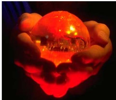
Figure 10: The Bitball – a ball with a tiny ‘cricket’ computer embedded inside it.
